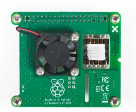
The Raspberry Pi PoE HAT is an add-on board for the Raspberry Pi 3 Model B+ (and later boards). It is used to power the Raspberry Pi via an Ethernet cable, provided that power-sourcing equipment is installed on the Ethernet network.
